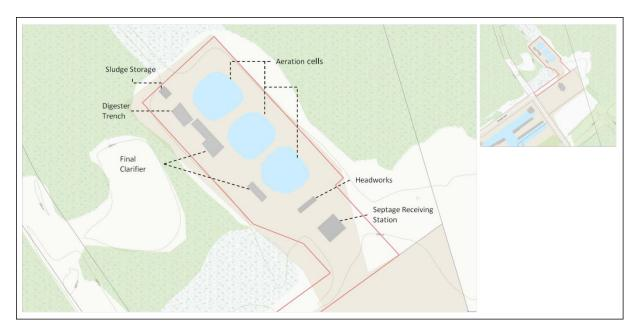
Figure 3: The Current Lagoon City Wastewater Treatment Plant Site Overview
