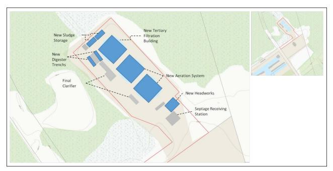
Figure 4: Site Overview with upgrades to expand plant capacity identified
